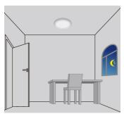
Light turns off when ambient lux level is higher than the preset lux amount
