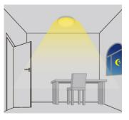
Light dims to stand-by level if no motion is detected after holdtime
