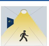
With insufficient ambient brightness, the light turns ON when motion is detected.
