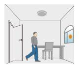
With sufficient daylight, even when motion is detected, the light remains OFF.
