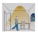
With insufficient daylight, when motion is detected, the light turns ON.
