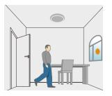
With sufficient daylight, even when motion is detected, the light remains OFF.
