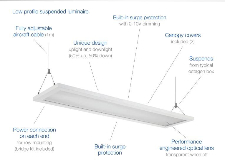
**Complete with:** 1m aircraft cable (x2), white canopy octagon cover, canopy covers (x2), and bridging kit (for row mounting)
