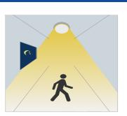
With insufficient ambient brightness, the light turns ON when motion is detected.
