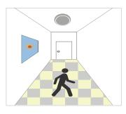
With sufficient ambient brightness, the light remains OFF when motion is detected.
