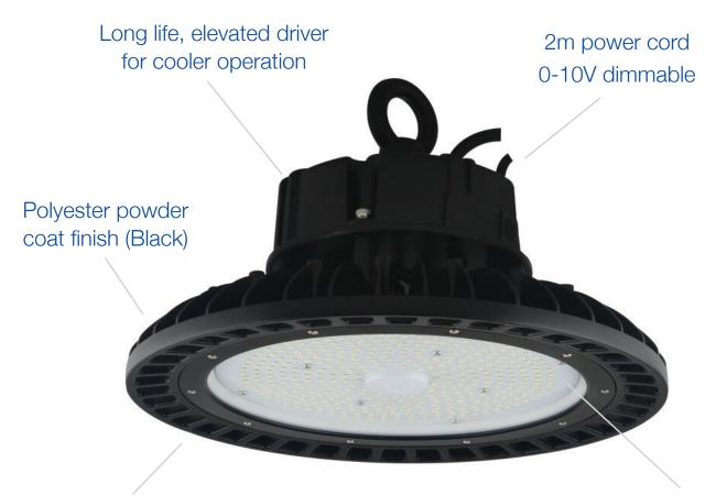
High grade aluminum body for superior heat dissipation 110° beam angle Shatter-proof polycarbonate lens
