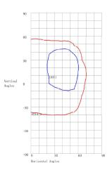
Maximum Candela = 42142 Located At Horizontal Angle =-55, Vertical Angle = 22.5 50% Maximum Candela = 21071 10% Maximum Candela = 4214 2
